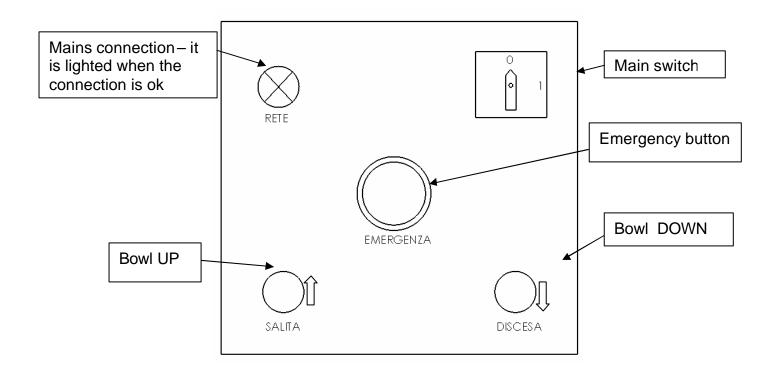
After switching ON the main switch verify the correct position of the bowl and **make sure the bowl is** securely fastened to the bowl holder.
