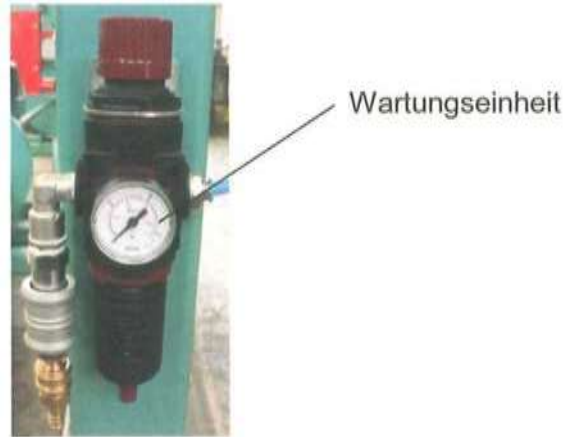
(Wartungseinheit = Maintenance Unit) Figure 23: Pneumatics
